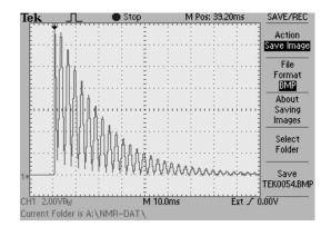
**Figure 6** – Oscilloscope Trace of Multiple Echoes
