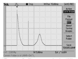
Figure 6a: Oscilloscope trace showing 180° pulse spike and spin echo.
