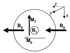
Fig. 3a Top view of the Sample showing the effect of a  $90^{\circ}$  pulse on the magnetization  $\mathbf{M}$  of the sample. The thermal equilibrium magnetization  $\mathbf{M}_0$  has been rotated to the transient  $\mathbf{M}_T$ .
