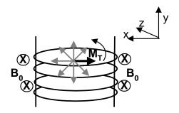
Fig. 3b Side view of the sample with,  $\mathbf{B_0}$ , the field of the permanent magnet, directed into the page. Following a 90° pulse, the net magnetization,  $\mathbf{M_T}$  precesses around  $\mathbf{B_0}$ .
