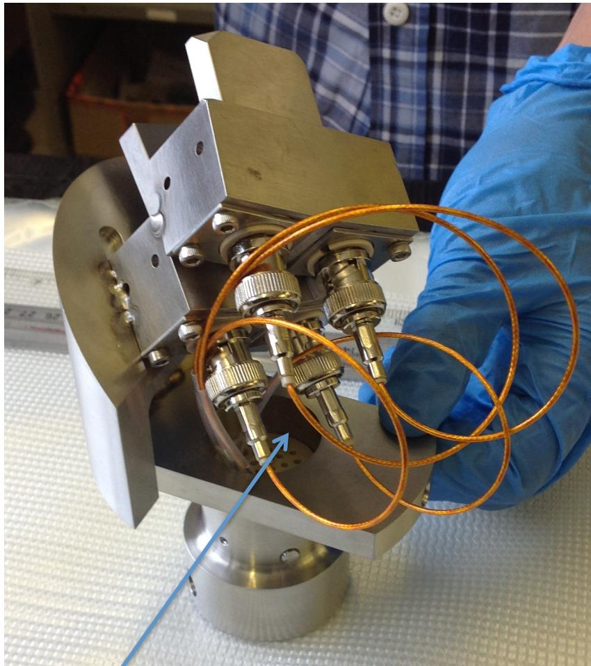
multi-pin probe head connector
